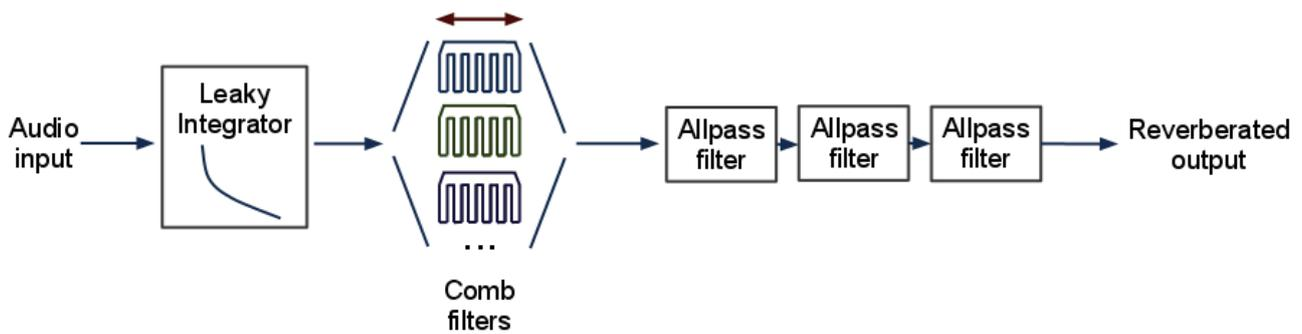
Figure 4: Signal chain of the reverberation instrument.
