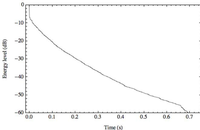
**Figure 2.** The energy decay as measured in the desiduous forest, exemplary for an outside space. The shown decay curves were determined using the backward integration method as proposed by Schroeder[4].
